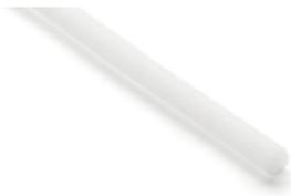
NOMATEC® Backer Rod XL round profiles are manufactured from closed cell, cross-linked polyethylen foam and are specially designed to backfill joints used with hot applied sealants. They provide the correct sealant reservoir configuration, control the depth and prevent bottom side sealant adhesion.
