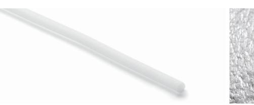
NOMATEC® Backer Rod XL round profiles are manufactured from closed cell, cross-linked polyethylen foam and are specially designed to backfill joints used with hot applied sealants. The provide the correct sealant reservoir configuration, control the depth and prevent bottom side sealant adhesion.
