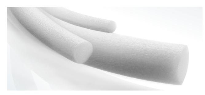
NOMATEC® Backer Rod XL round profiles are manufactured from closed cell, cross-linked polyethylen foam and are specially designed to backfill joints used with hot applied sealants. The provide the correct sealant reservoir configuration, control the depth and prevent bottom side sealant adhesion.
